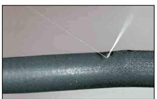
Fig 15 - Leak in transfer hose
