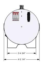
4600L Double Wall Tank - Integral Contained
