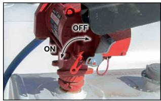
Fig 20 - Pump operation
