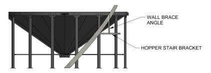
3. Locate the ideal locations for the remaining wall brace angles. Line up the hopper stair brackets accordingly to fit to the wall brace angles.
