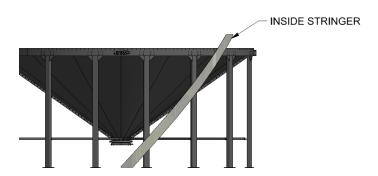
2. Install the top wall brace angle. Attach the top of the wall brace angle to the bolts on the top hopper band, and the bottom of the wall brace angle to the hopper stair bracket. The hopper stair brackets can be attached to the legs of the hopper with U-bolts.
