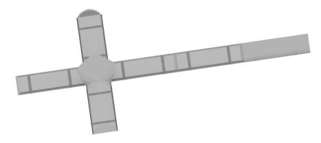
Straightly place the Aeration tubes as drawing shown, and overlap 2" to each other.
