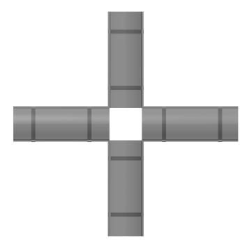
Place the Center [166683] on the top of the four Aeration tubes. The assembled joint should look like shown on picture. There are no screws necessary for assembly.
